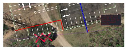
Figure 2 – Existing 525 mm pipe shown in purple. The red line indicates the hypothetical carpark boundary to avoid impacting trees No. 14, 15 and 16. The blue line illustrates the stormwater connection into existing pipe.
