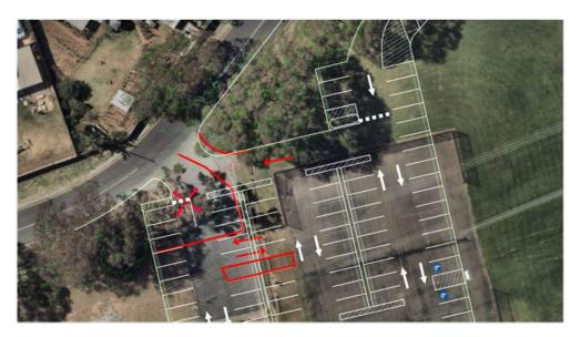
Figure 1 – Red lines illustrating the constraints involved in keeping tree No. 12 and existing driveway
