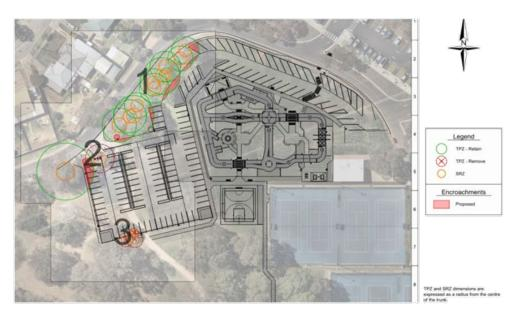
Figure 4 - Carpark geometry and impact on existing trees
