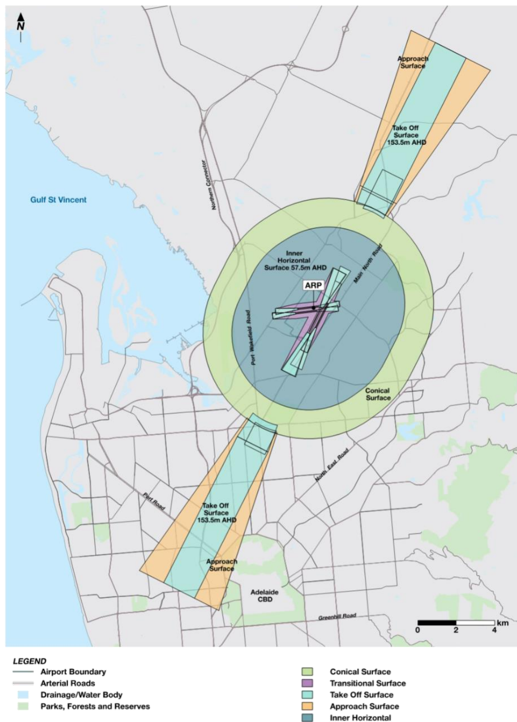
Figure 12.4: Obstacle Limitation Surfaces (OLS) plan for Parafield Airport
