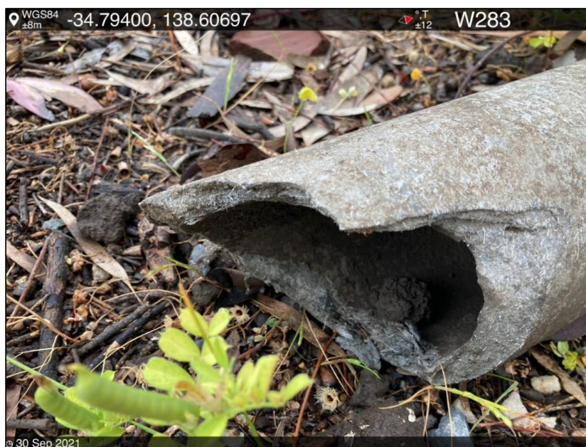
Photo 7: Potential ACM piping, northern boundary of site
