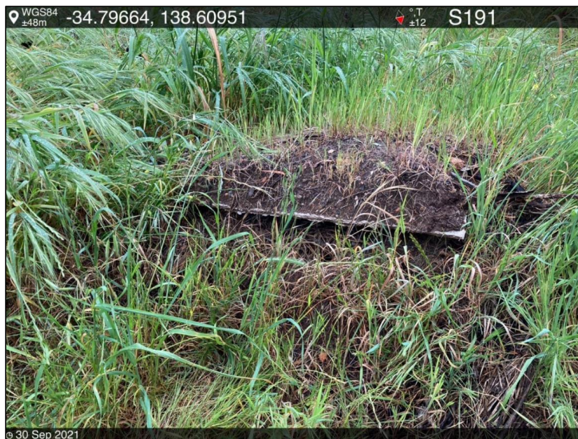
Photo 6: Soils on top of suspected asbestos cement sheeting near the southern boundary of site
