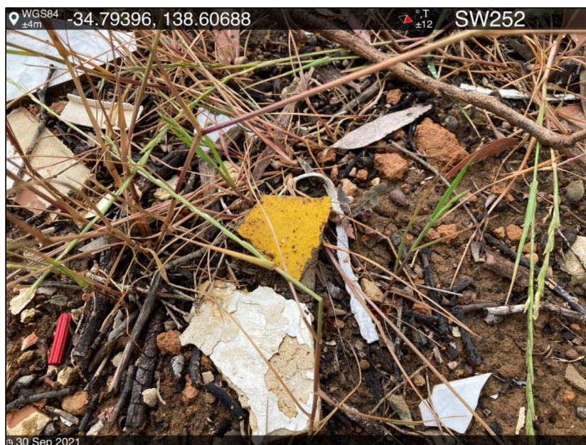
Photo 8: Example of potential ACM near the northern boundary
