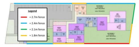
With the acoustic recommendations implemented the highest predicted outdoor sound pressure level at any residential will be 50 dB(A) and therefore is in accordance with the assessment criterion from the WHO guidelines and shall not unreasonably impact adjoining properties.
