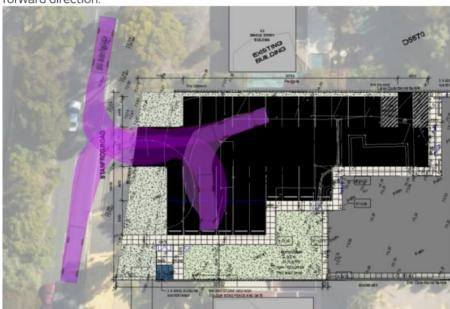
Figure 2 - MRV turning movements into and out of the site
