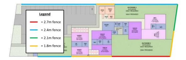
Where a retaining wall is proposed, such that the outdoor play area is lower than the height of the adjacent residence, the criteria can be achieved with a lower fence height. The fence height may therefore be reduced by 0.3 multiplied by the retaining wall height.
