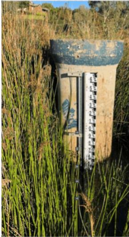
Photo 2 : Survey staff used to note water level – Photo date 25 October 2021
