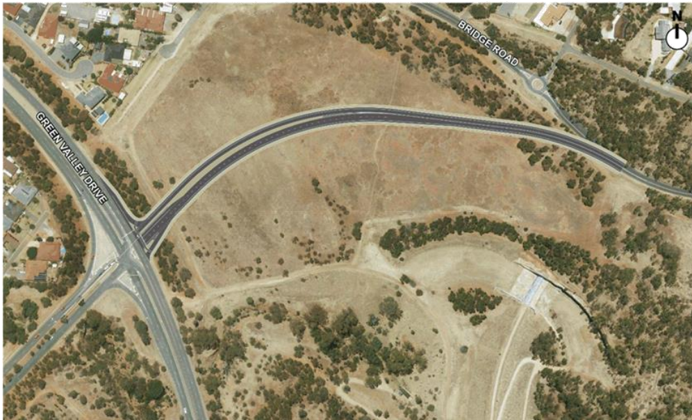
Figure 4.8 Green Valley Drive realignment to Bridge Road
