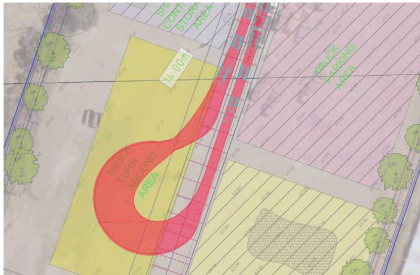
Figure 4 - B-Double (26 m turnaround manoeuvre)
