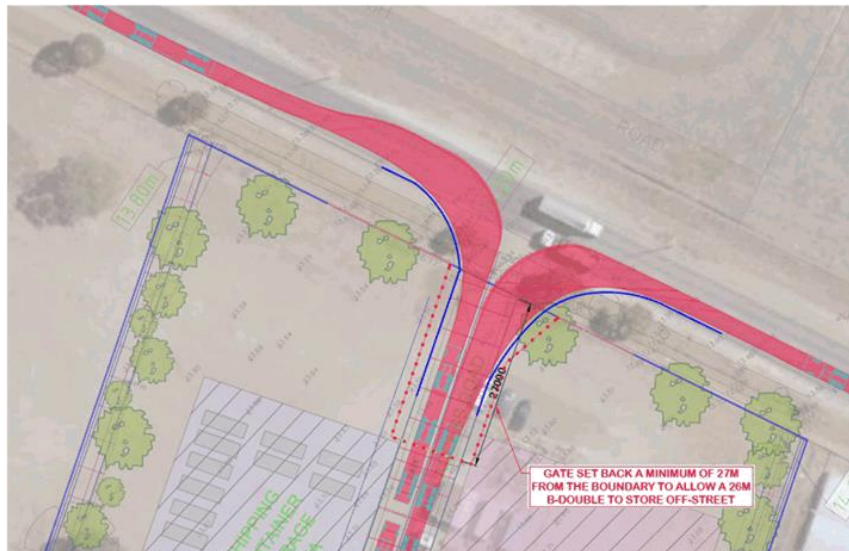
Figure 3 – Simultaneous B-Double turn paths at the Edinburgh Road access point
