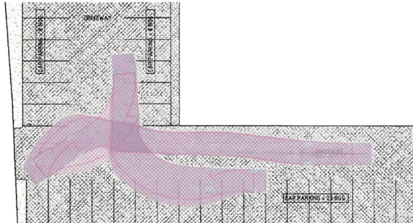
Figure 3 – An 8.8 m refuse collection vehicle entering and exiting the site in a forward direction
