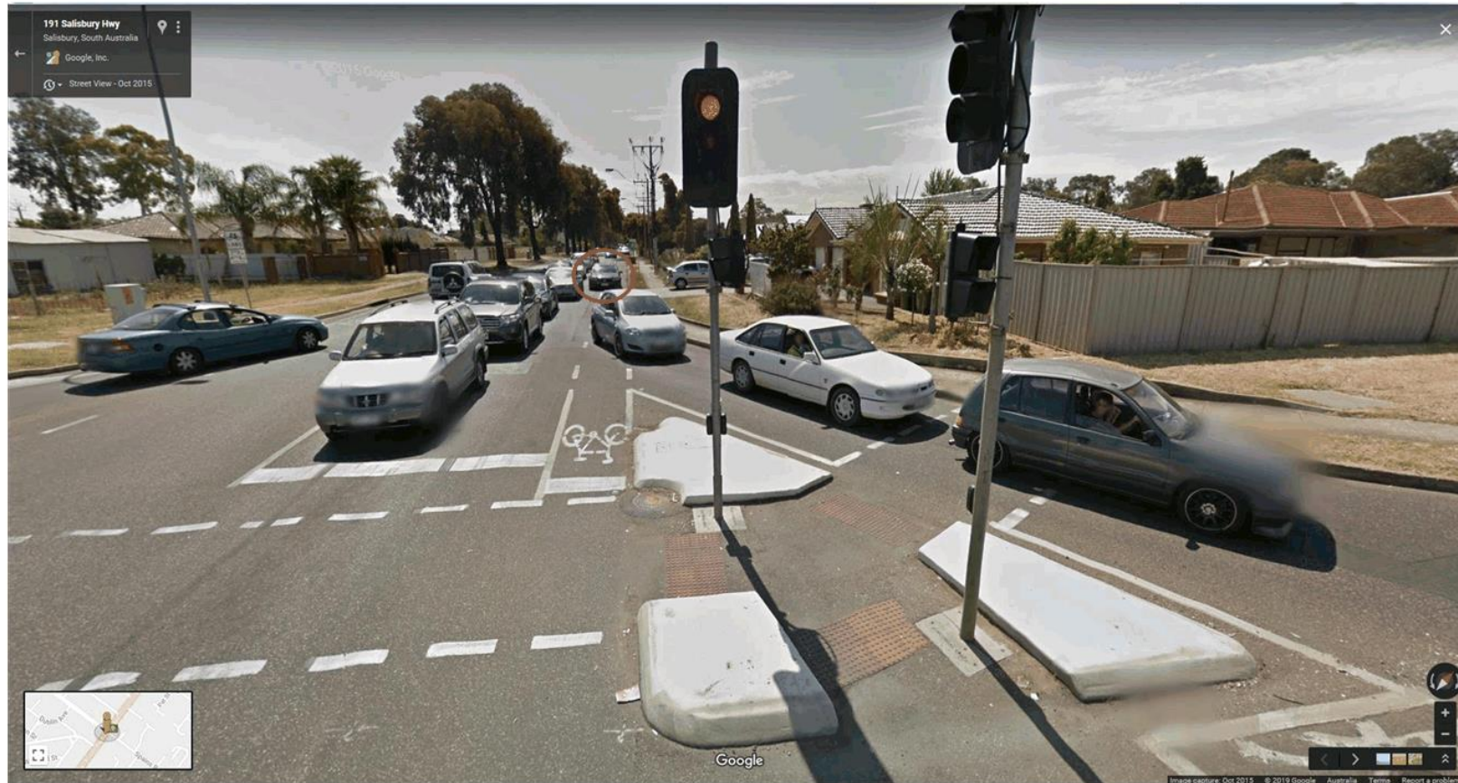
Vehicle seeking to turn left (circled in red) must queue behind through lane traffic as there is insufficient clearance
