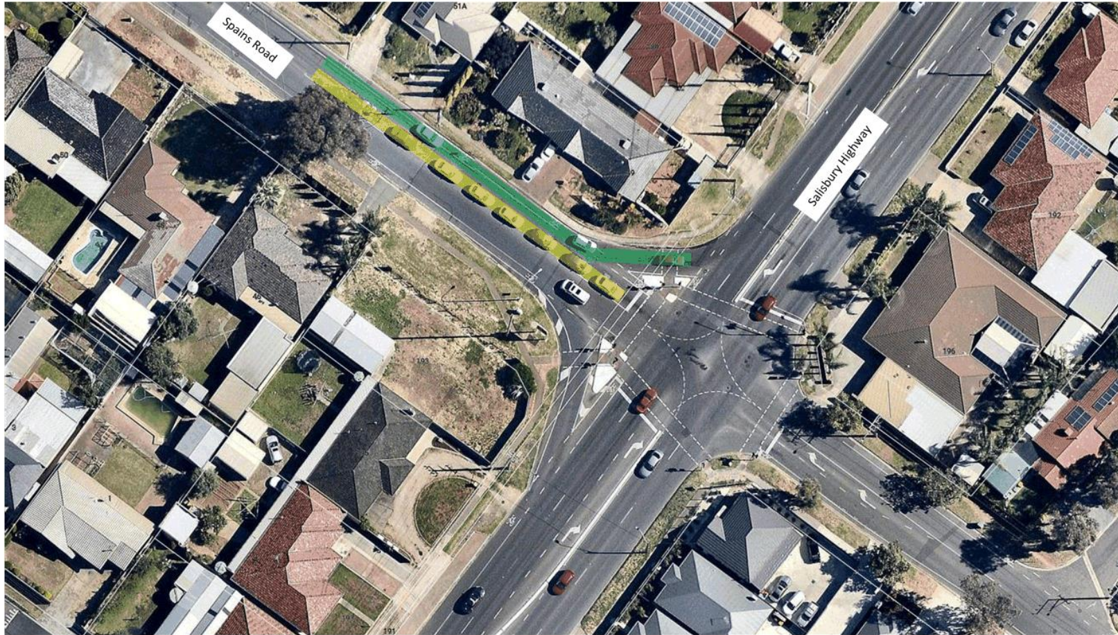
Vehicles queued in the through lane (highlighted in yellow) are straddling the centreline which provides sufficient clearance for vehicles seeking to turn left (highlighted in green) to overtake and access the left-turn slip lane
