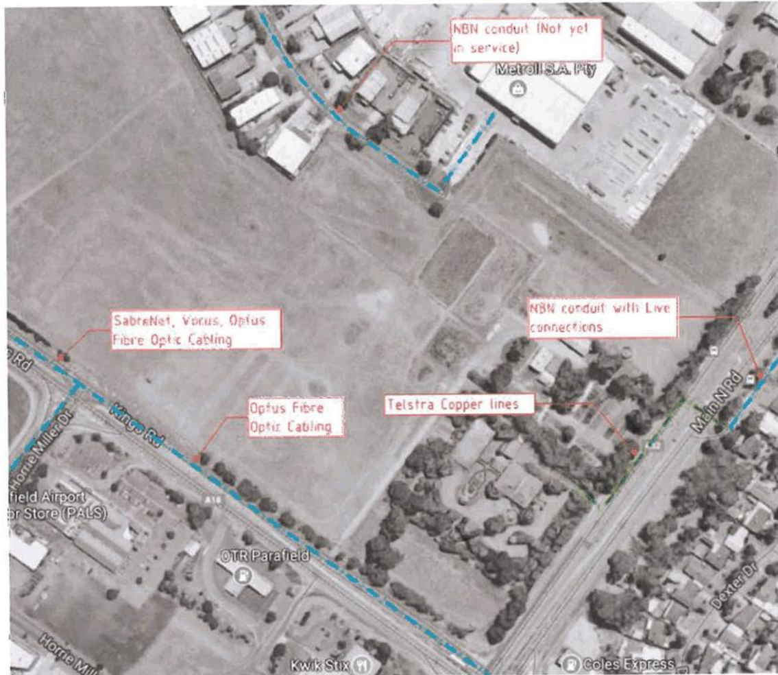
Figure 7: Communications Inground Infrastructure
