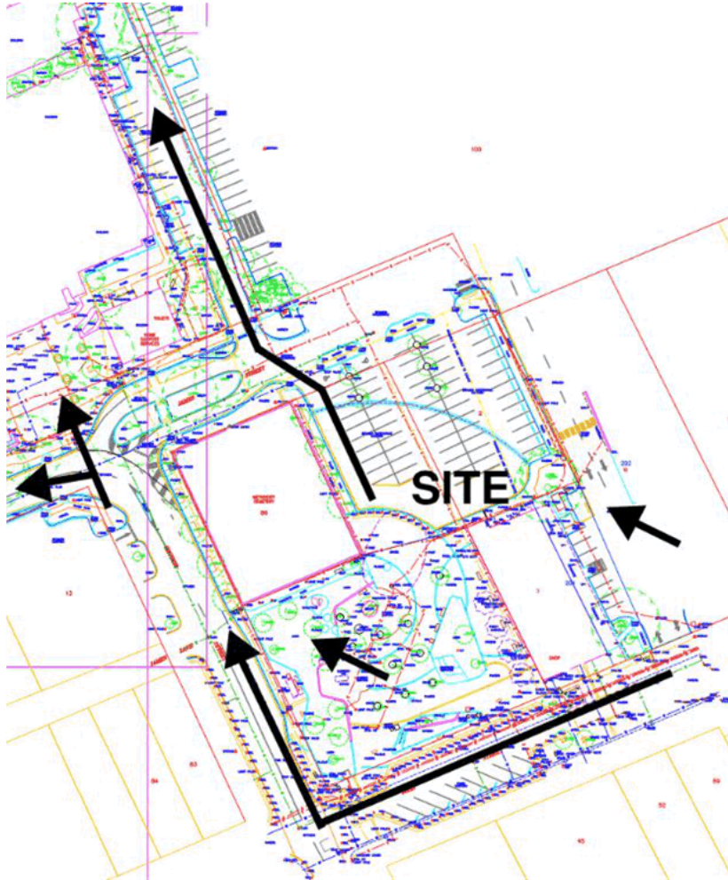
Figure 5.1 Existing Major Stormwater Overland Flow Paths
