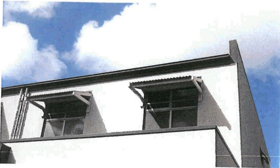
Above and below - Alternative upper level window opening design for varied upper level north elevation for units 1-5 allowing for lower panel to be obscure glazing, with upper portion restricted opening. Example from approved Distinctive Homes development, Joseph St, Salisbury (final detail of glazed panel proportions may not match this exactly).
