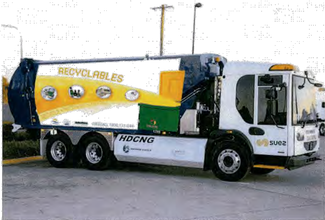
New Suez Truck using High Density Compressed Natural Gas as a Fuel Source
