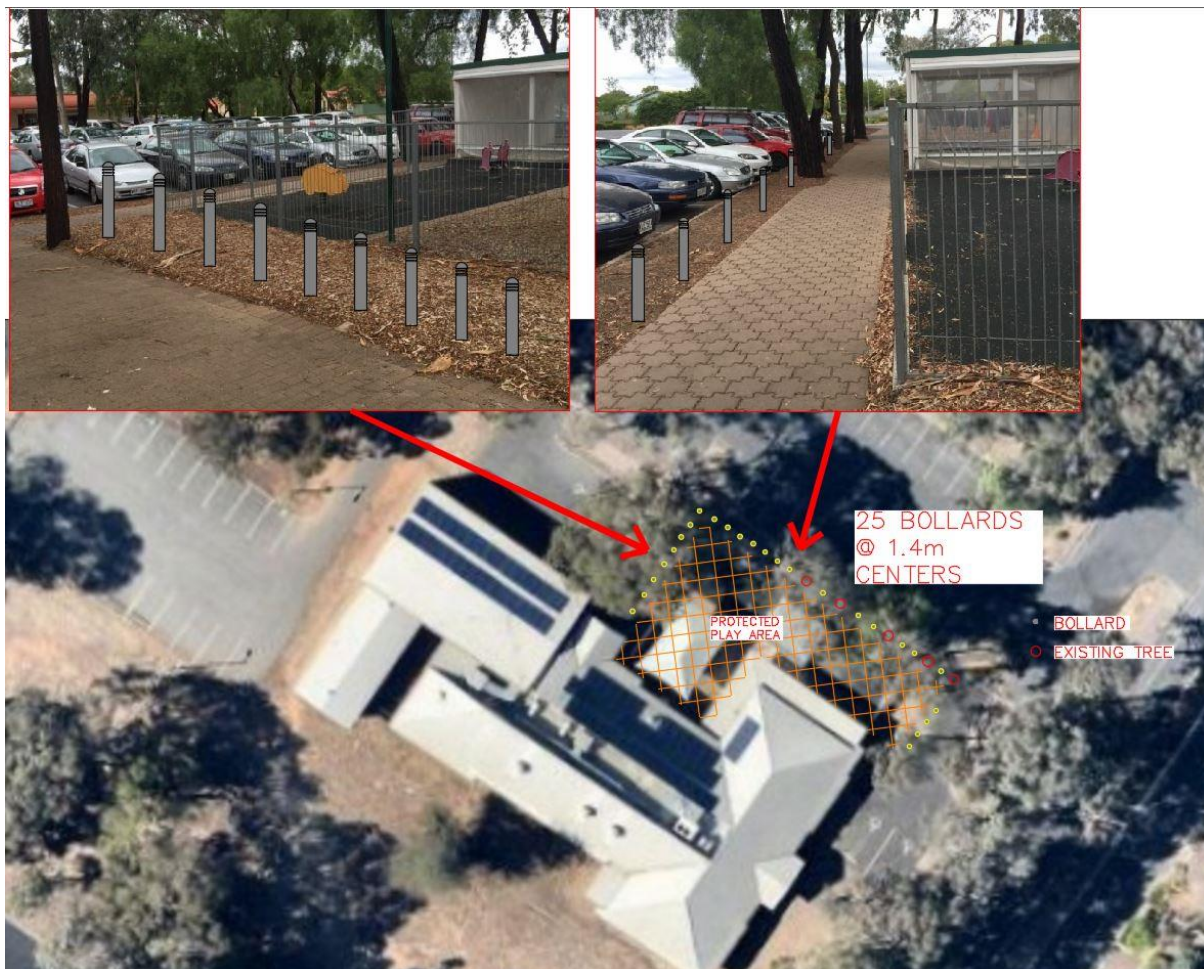
SITE LAYOUT PLAN FOR THE INSTALLATION ENERGY ABSORPTION BOLLARDS AT THE BAGSTERS ROAD COMMUNITY CENTRE AT SALISBURY NORTH
