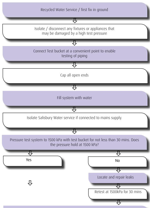
If possible, ensure the Salisbury Water system is pressured during concealment prior to commissioning.
