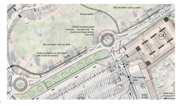
To enable coaches and long trailers to effectively navigate to the boat ramp and new bus layover area, a slip lane is proposed for the intersection of Mangrove Street and St Kilda Road.
