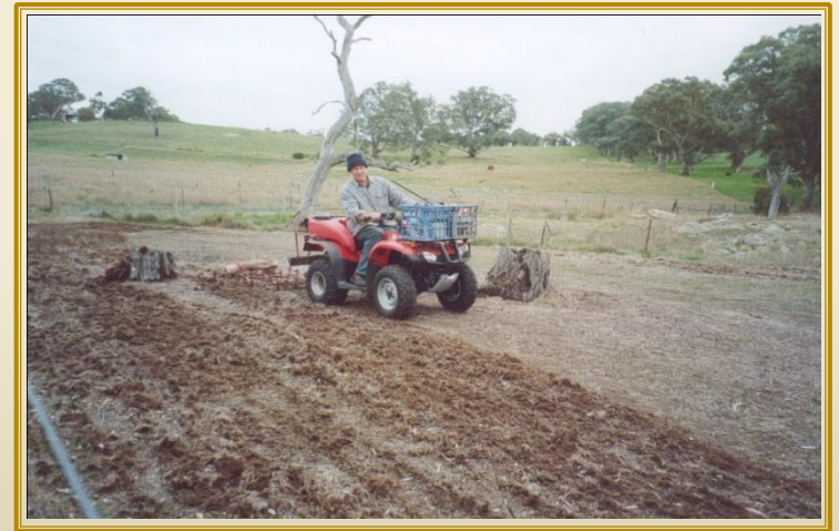
Dragging a simple 20 spike harrow
