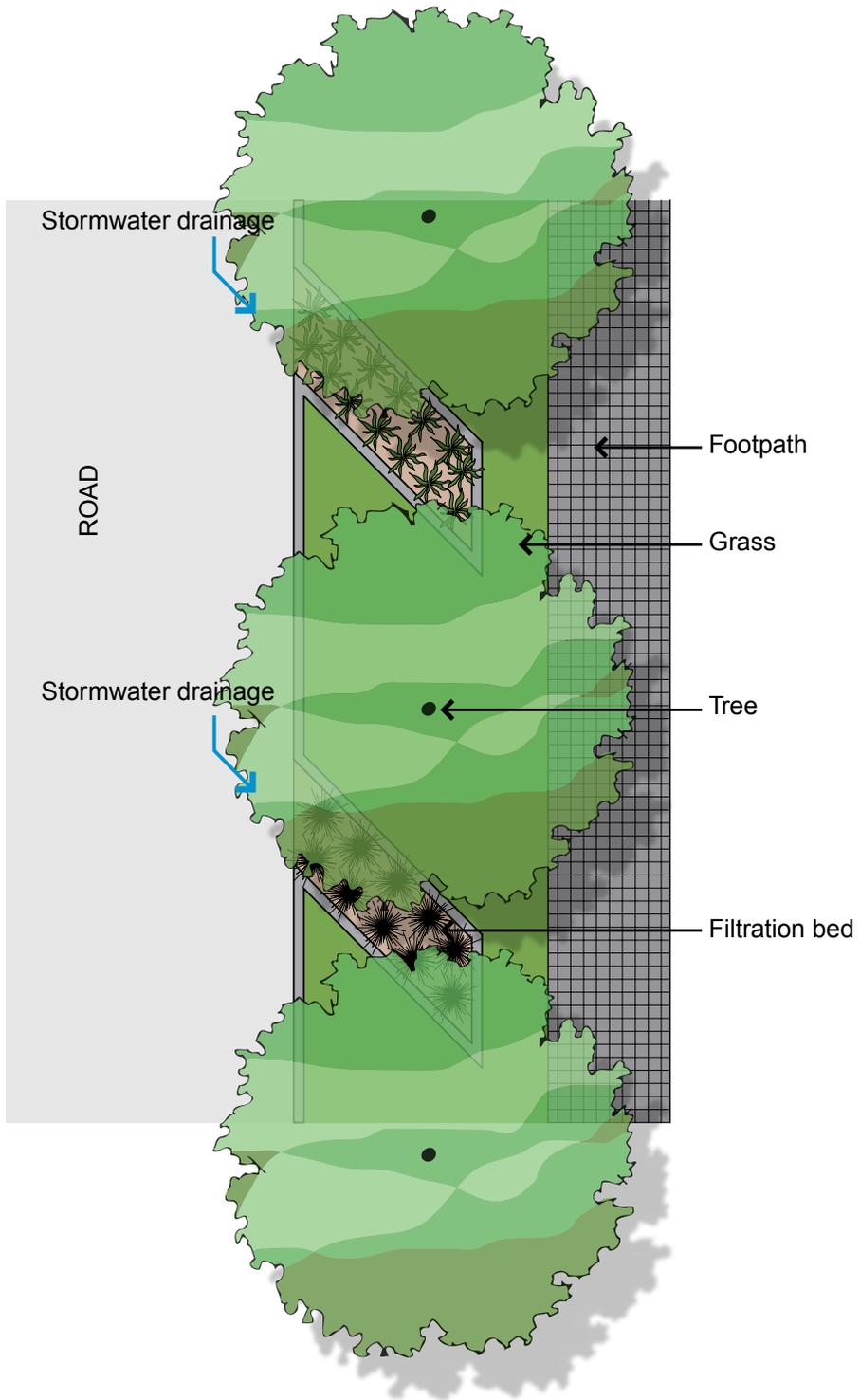
Figure 5.13: detention swale - local street plan 02
