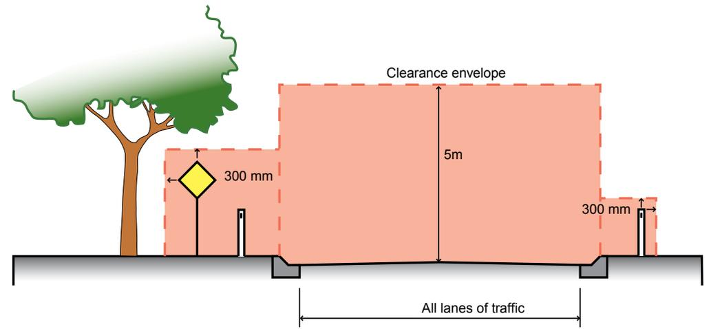
Figure 5.3: secondary clearance zone
