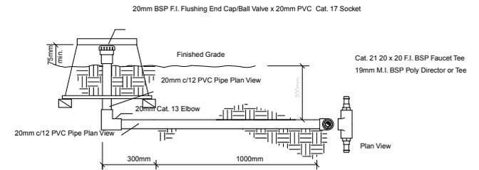
Flushing Valve Assembly
