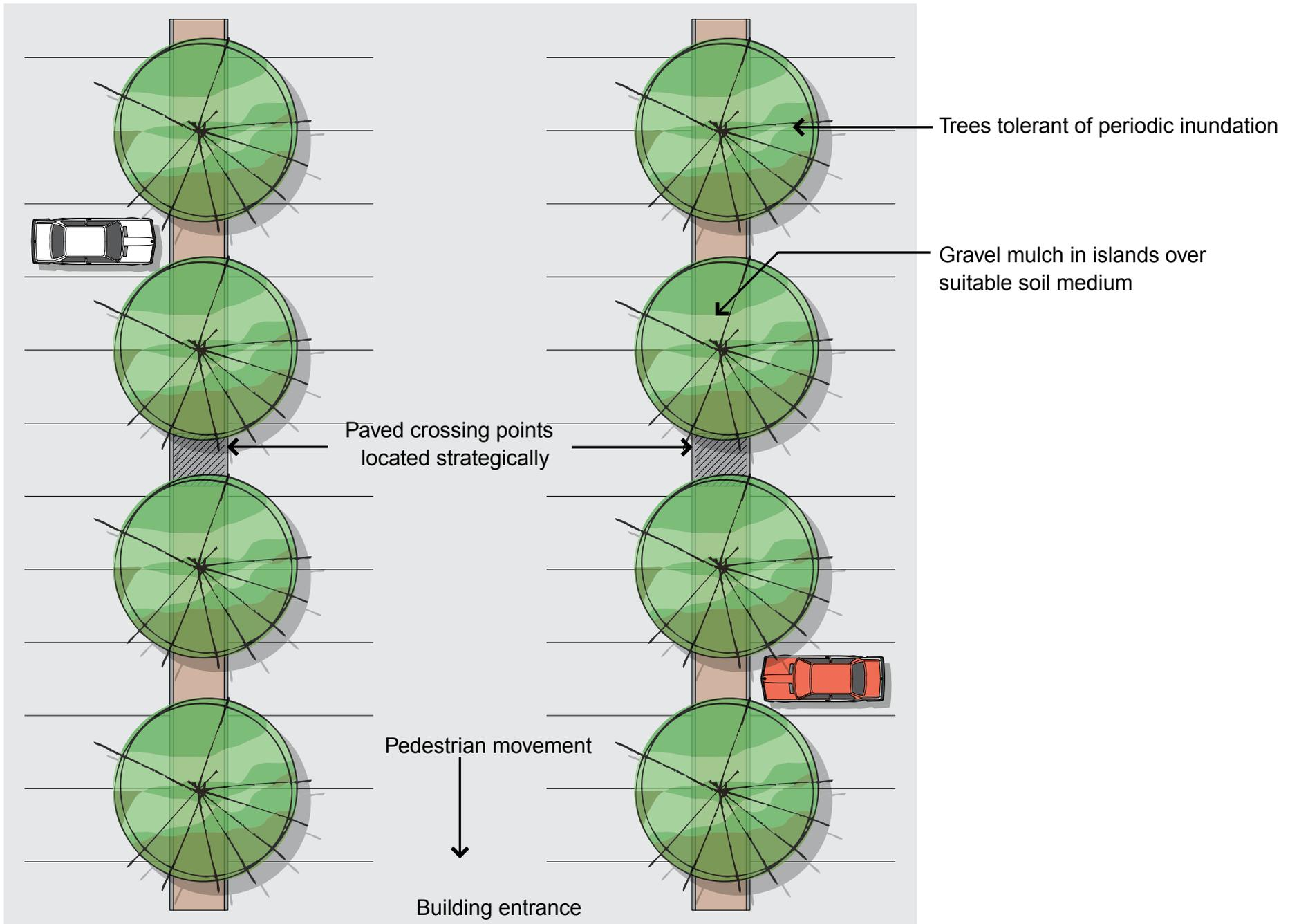
Figure 6.2: detention swale car park plan 01
