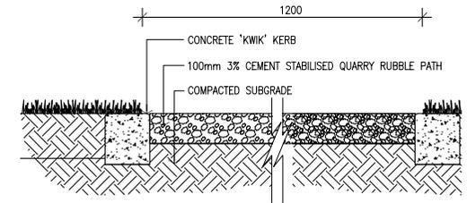
TYPICAL CEMENT STABILISED QUARRY RUBBLE PATH
