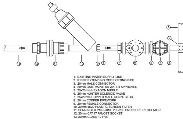
Drip Irrigation Valve Assembly
