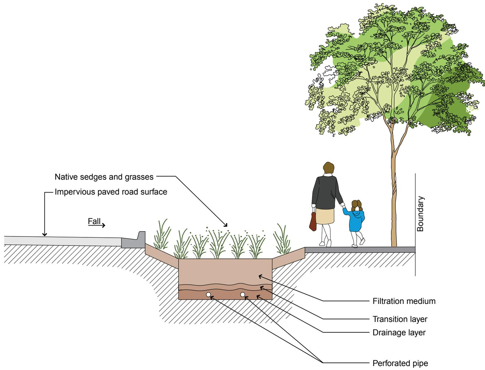
Figure 5.11: detention swale - local street section
