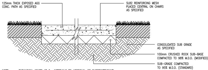
EXPOSED AGGREGATE CONCRETE PATH
