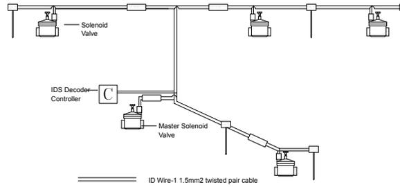
Decoder Wiring Schematic NTS
