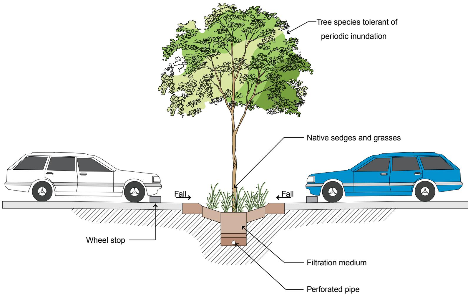
Figure 6.1: detention swale - car park section
