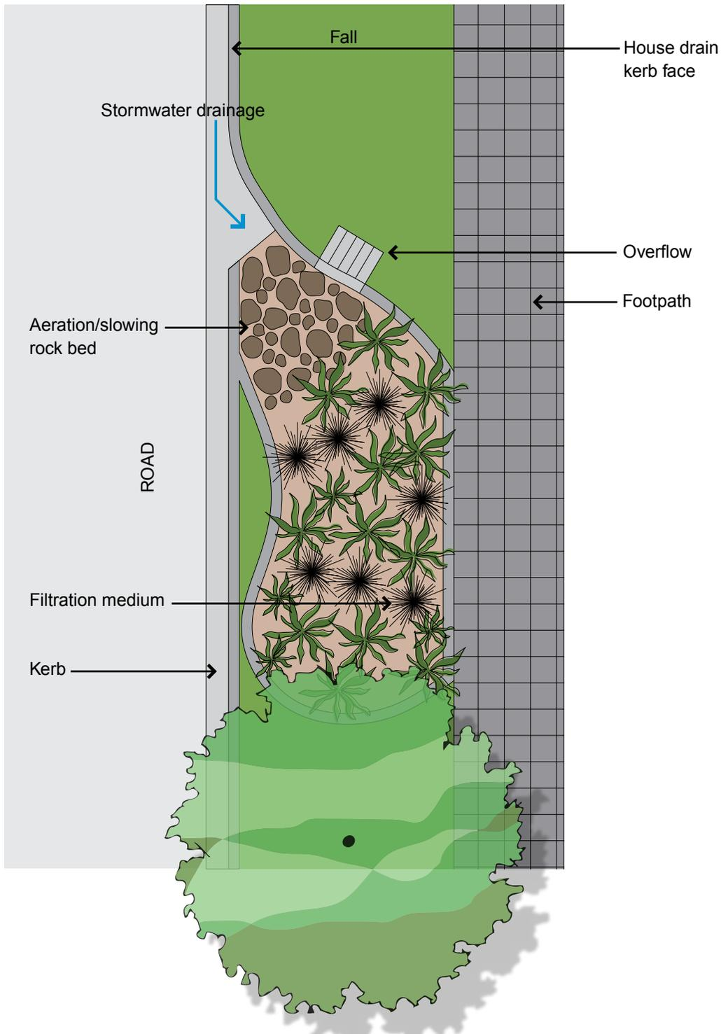
Figure 5.12: detention swale - local street plan 01
