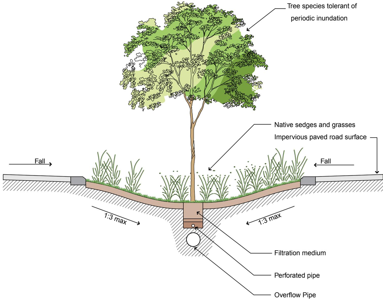
Figure 5.10: detention swale - median
