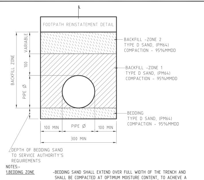
MINIMUM COMPACTION OF 95% MMDD. BY TAMPING, ROLLING AND/OR VIBRATING.SAND SHALL BE PLACED IN LAYERS NOT EXCEEDING 150mm COMPACTED THICKNESS (200mm UNCOMPACTED).
