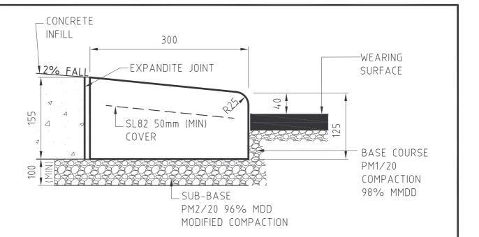
70mm MOUNTABLE KERB FOR A FULLY MOUNTABLE CENTRE ISLAND OF A MINI ROUNDABOUT
