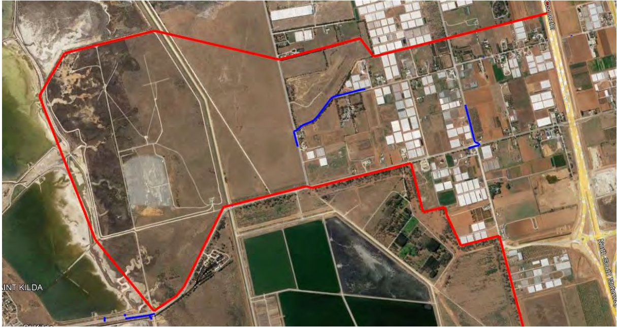
Figure 15: Stormwater Precinct 4 Existing Stormwater Drainage Infrastructure
