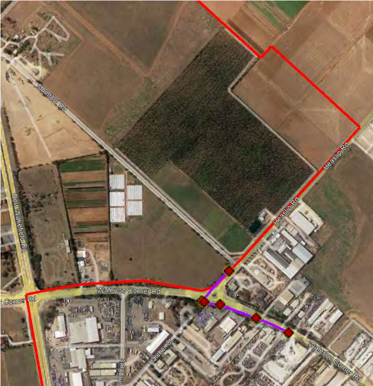
Figure 26: Precinct Area 3 - Existing City of Salisbury Recycled Water Infrastructure
