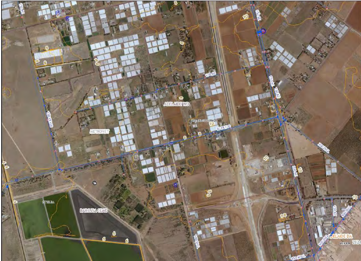
Figure 21: Precinct Areas 2, 3 & 4 - Northern- Existing SA Water Potable Water Infrastructure
