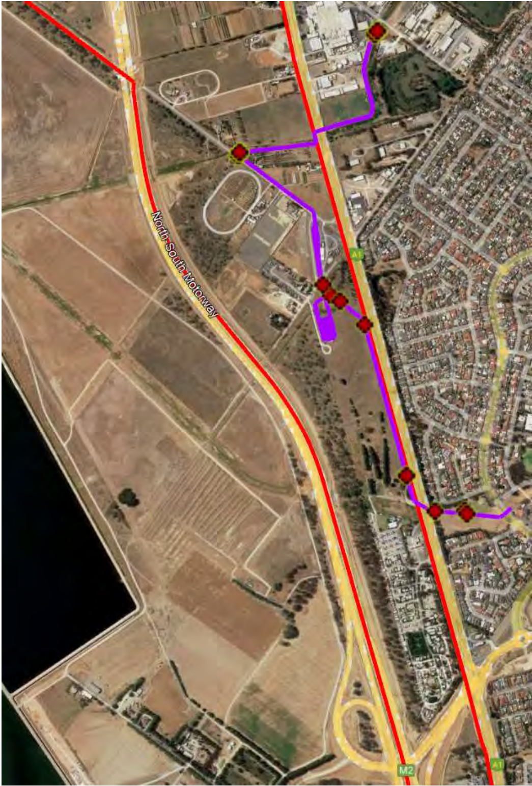
Figure 25: Precinct Area 2 (2A & 2B) - Existing City of Salisbury Recycled Water Infrastructure
