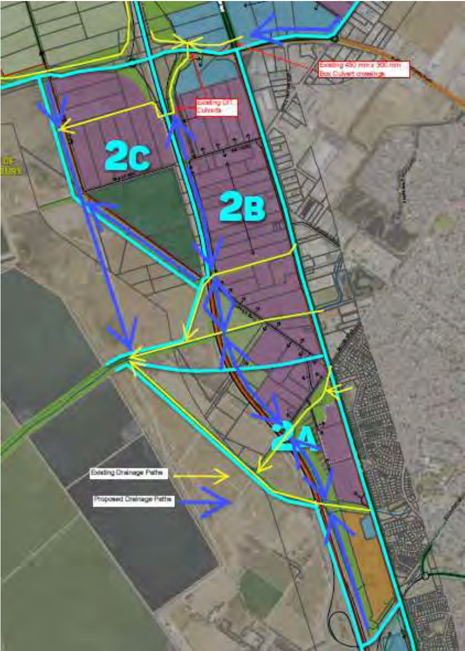
Figure 8: Stormwater Precinct 2 Drainage Paths
