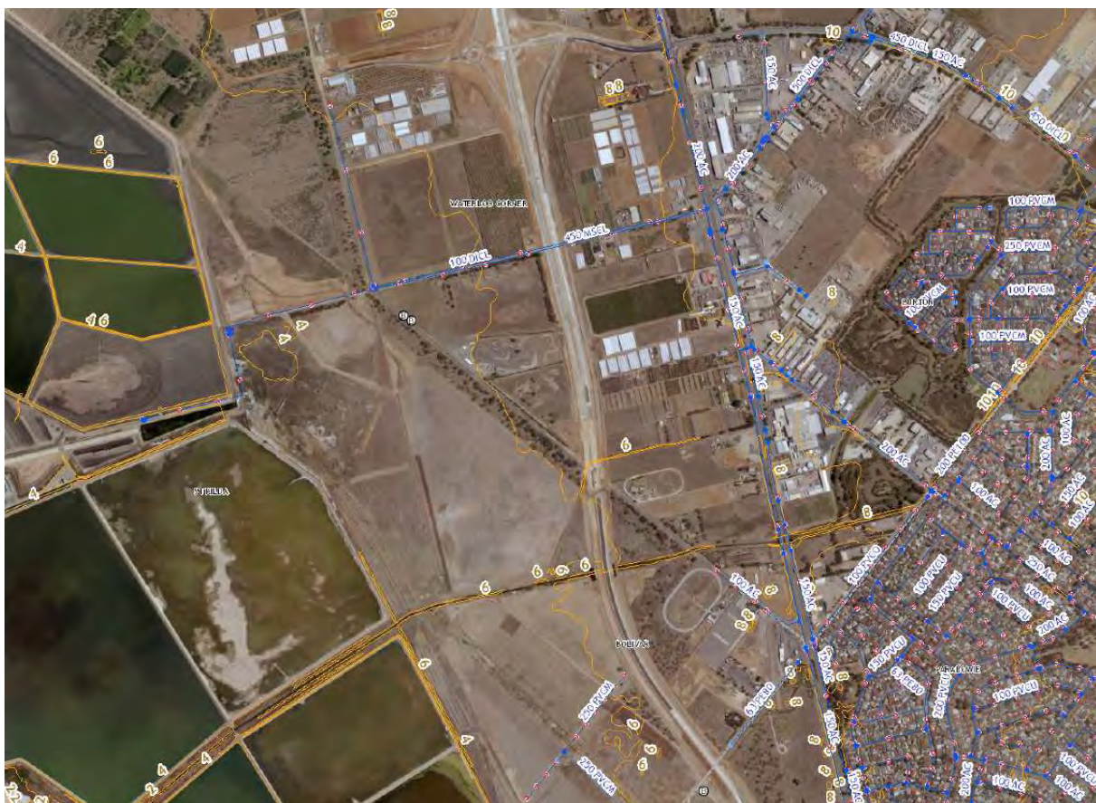
Figure 20: Precinct Areas 2 & 4 - Central - Existing SA Water Potable Water Infrastructure
