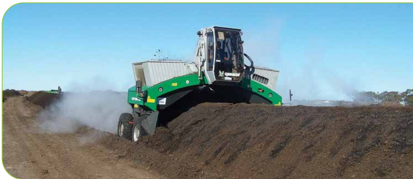
Peats Composting Windrow Turner turns FOGO items into high performance organic soil conditioner.
